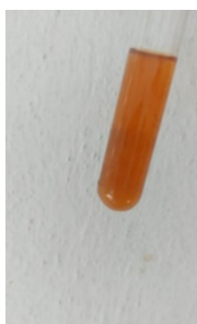
Figure 33: Test for Chloride
